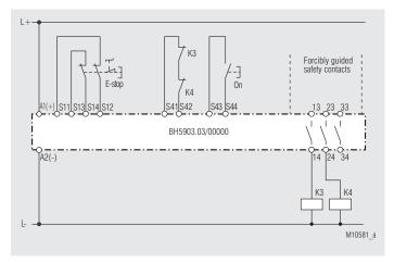
BH 5903 with external contact reinforcement
