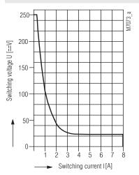
safe breaking, no continuous arcing under the curve, max. 1 switching cycle/s
